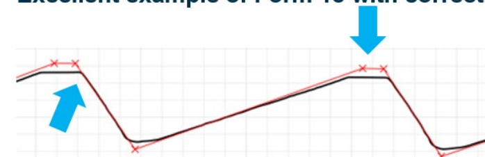
Land not finished – should have been had 1 more pass.
