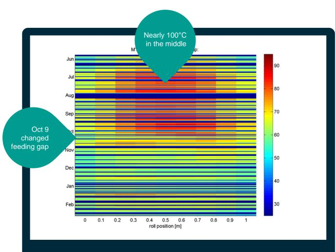
High temperature difference between left/right side of the roll compared to the middle of the roll.
