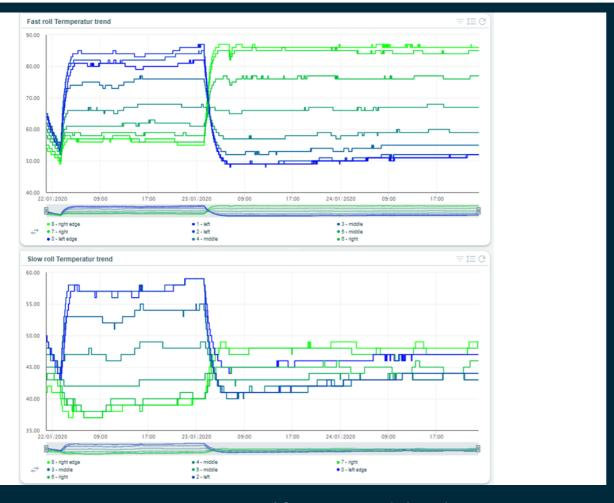
High temperature imbalance over 30°C between left (blue) vs right (green) side of the roll.
