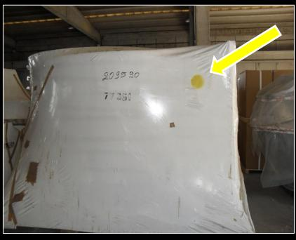
**Before shipping departure**, every single package delivered is assigned considering the colour used for specific machines on the layout drawings
