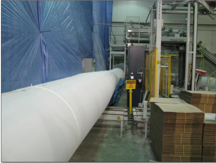
A temporary Poly-tarp – no sealing
